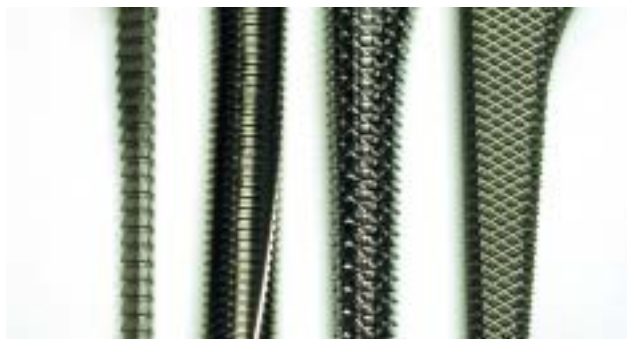
Figure 4, picture of several other modern broach tooth patterns
