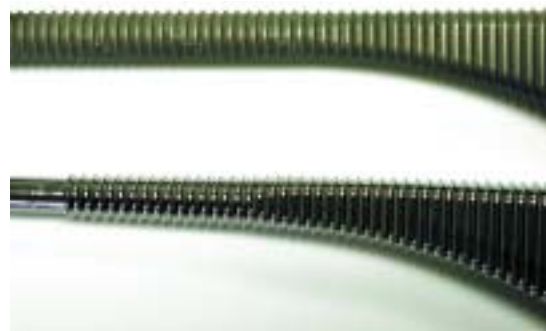
Figure 5; Close-up photos of a milled vs. ground broach or reamer
