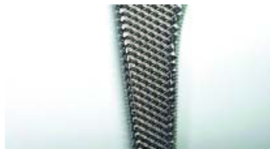
Figure 3. Diamond Tooth Pattern
