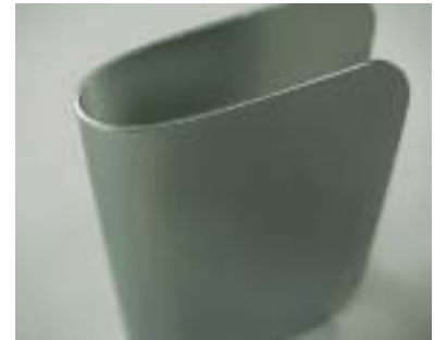
Figure 3. Photograph of the outer area of the 180° bend of the AISI 304L stainless sample coated with low friction chromium. There is no evidence of crazing, peeling, or cracking of the coating from the base metal. 4X Magnification.
