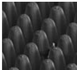
Laser Texturing of Graphite (75 µm diameter x 200 µm tall columns)
